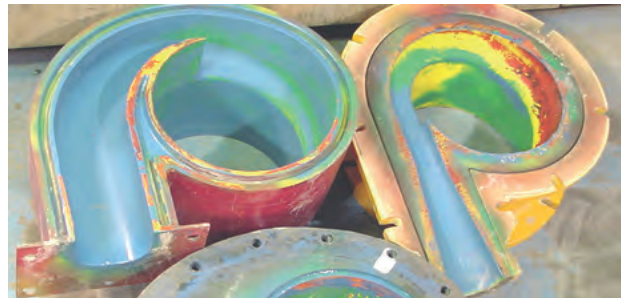
Paint wear test: gMAX® vs. outer wall tangential
